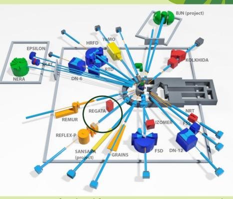
Layout of pulsed fast reactor IBR-2 at JINR in Dubna
